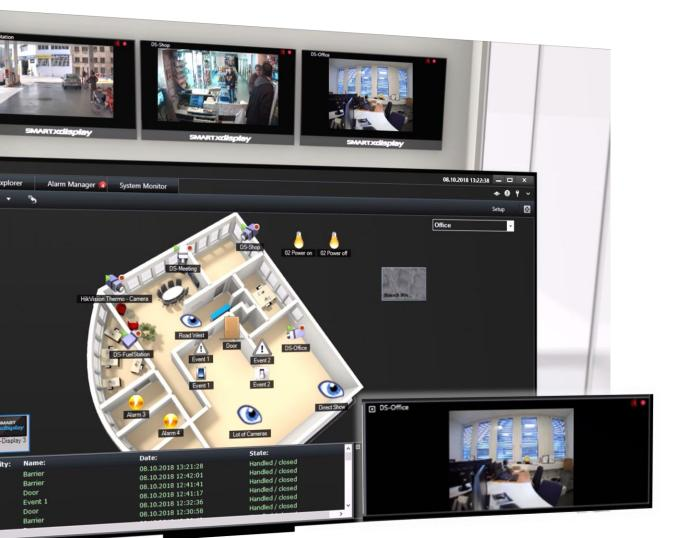
The focus window displays the camera that currently has the focus.
