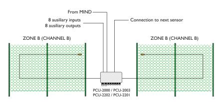
The sensor provides a series of NC contacts, via terminal blocks, for the signals of Pre-alarm, Alarm, Cut and Short for channel "A" and channel "B" and, in addition, the Fault and Tamper signals.
