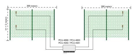
If the sections to be protected were sequential, the length of the two outer sections may be up of 150m since the beginning of the distant sections will be connected to the analyzer through a non sensitive cable with a length equal to those of the two sections closest to the analyzer.
