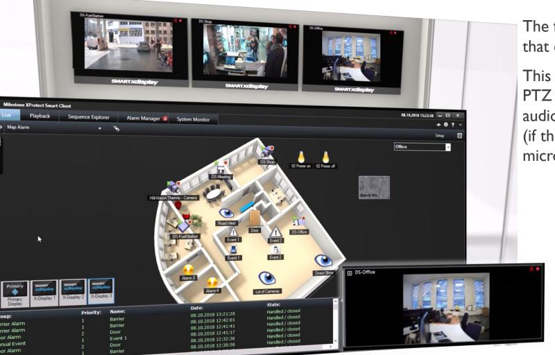
The focus window displays the camera that currently has the focus.
