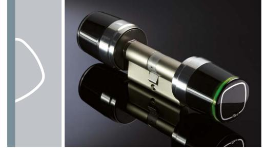
The **Libra Smart** electronic cylinder can be easily installed on both new and existing doors. It can be used with any type of mechanical lock compatible with the European cylinder, and doesn't require any wiring so it's simple to switch from a mechanical cylinder to an electronic one.
